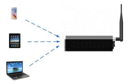
**Indirect Mode**: Configure an external router for a SBPro-HD and users can access the SBPro-HD by connecting the external router. If an external router is configured for multiple SBPro-HD units, a LAN can be created. Users can access any of the SBPro-HD via the LAN
